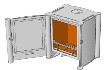
1. Stove shown in woodburning mode. Lift out woodbar and remove base bricks.
