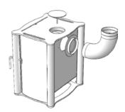
Figure 4 1. top outlet 2. rear outlet
